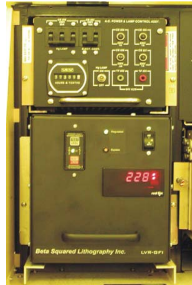
GFI-LVR Installed in Machine under A.C. Power & Lamp Control Ass'y.
